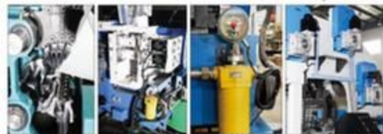
碳素纤维针床 Carbon fiber bed 电子牵拉装置(选装) Servo electronic draw-off 油压报警装置 Oil pressure warning device 电子送经装置 Electronic let-off device
