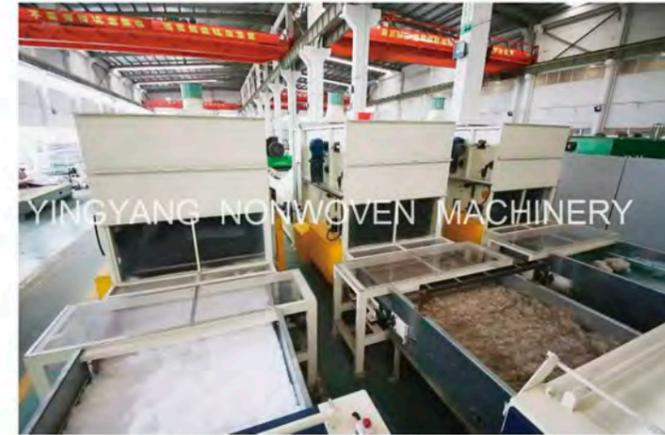
▼ Needling or thermal-bonding oven after carding and cross lapping system
