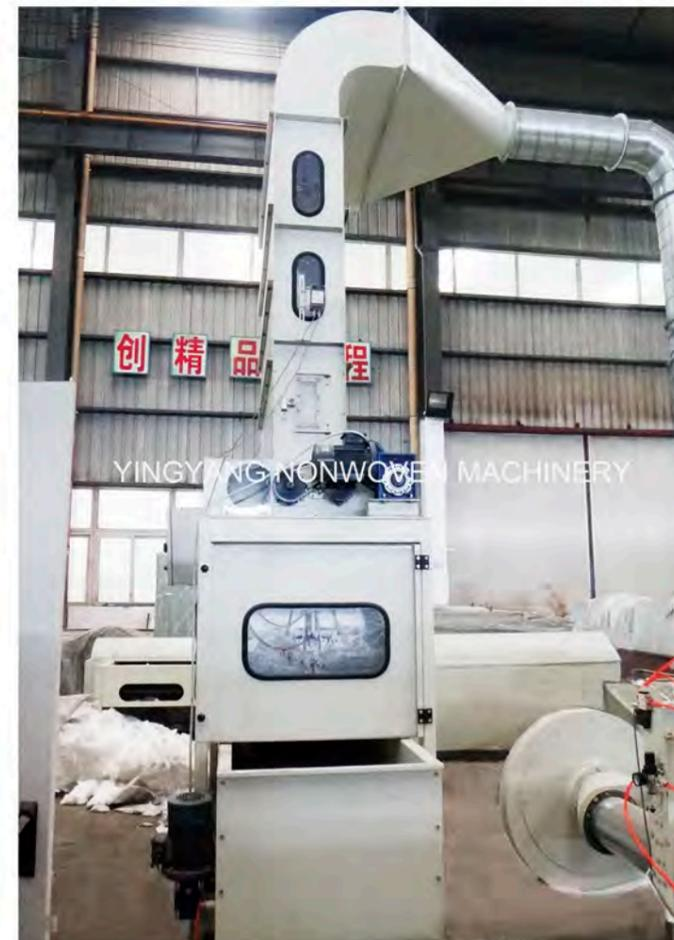
▲ Electronic weigh pan to control the accurate stuffing of each pillow
