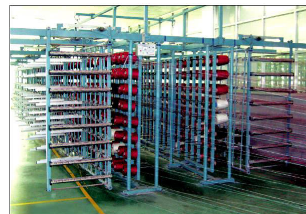
回转 V 型筒子架 rewind V-shaped bobbin creel
