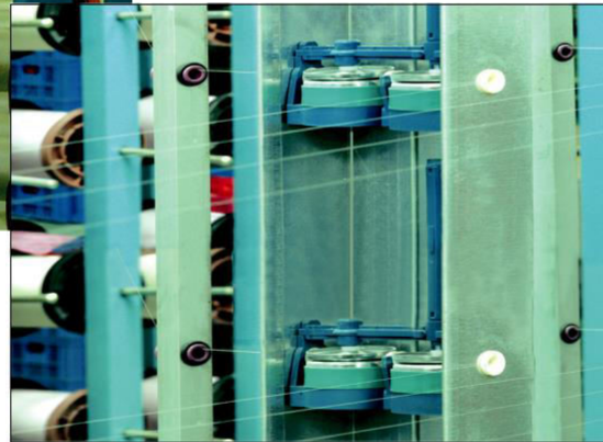
双盘无立柱积极转动式张力器 Double tray with no upright post, positive driving typed extension device
