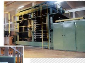
Advanced electronic yarn storage shelves allow operator to make direct input on the operating panel of headstock according to tensions of different yarns.
