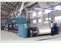
This series are mainly used in association with shuttleless loom for sizing warp of high-density, and broad cotton fabric, cotton-chemical fiber blend fabrics, linen and linen-chemical fiber blended fabrics.
