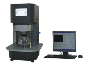
Determination pressure for a variety of fabrics, including knits, woven fabric, non-woven fabric, laminated fabric and other craft-made variety of fabrics, in standard conditions or under wet bursting strength and bursting dilation.
