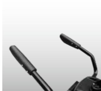
■ Standard equipped with armrest, when put down armrest, max. driving speed is 3.0km/h; when close up armrest, max. driving speed is 6.0km/h
