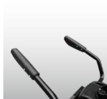
■ Standard equipped with armrest, when put down armrest, max. driving speed is 4.5km/h
