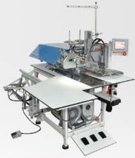
New-tech 2050/5 BREAST WELT POCKET AUTOMAT Capacity: 900-1000 Breast Welt Pockets / 8 Hours
