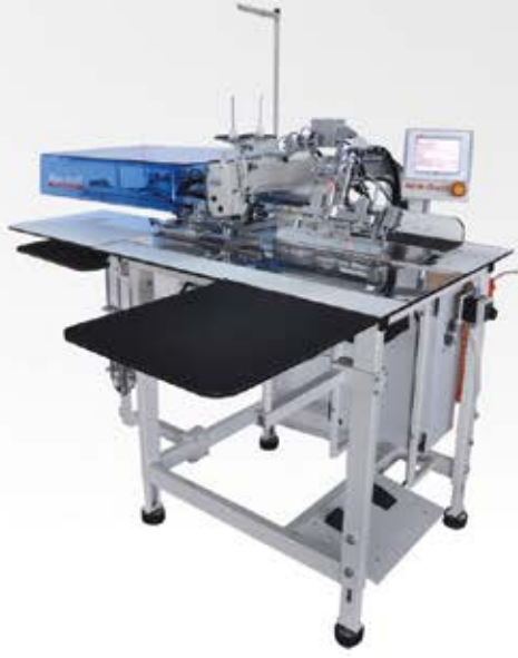
New-tech 2600/1 POCKET FACING AUTOMAT FOR TROUSERS AND JACKETS (LOCK STITCH) Capacity: 4000 Facings / 8 Hours
