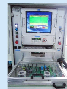
Automatic PCBA ATE test platform
