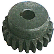
5 电机齿轮 (2°22′) Worm driving gear
