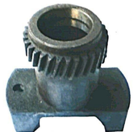
17 行星轮架(3"31') Revolving arm for differential
