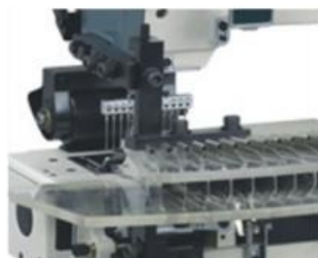
VC8008-12064P/VPT 12-needle half cylinder type back and forth Driving double chain stitch machine
