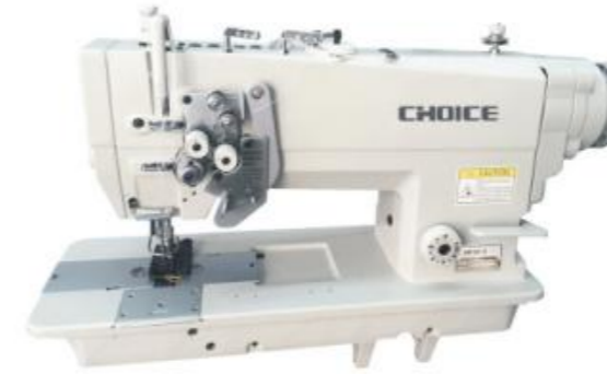
GC845-D / GC875 -D Direct drive 2-needle lockstitch small / big hook split needle bar
