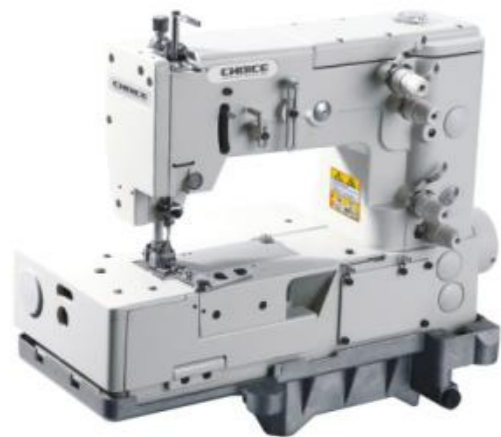
GC1302-4W / GC1803-1S Double needle 2/3/4 points picot/ facot chain stitch sewing machine
