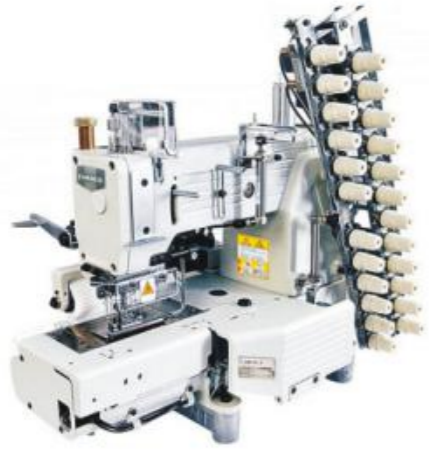
GC4412P/PUT/PL/DD Computerized 12N cylinder bed chain stitch machine with auto trimmer and auto foot lifter with roller set
