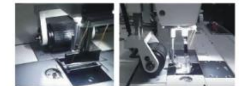
GC8423T Direct-drive double needle lockstitch sewing machine for waist banding, small hook, flat rear puller , width 36mm, 38mm, 40mm
